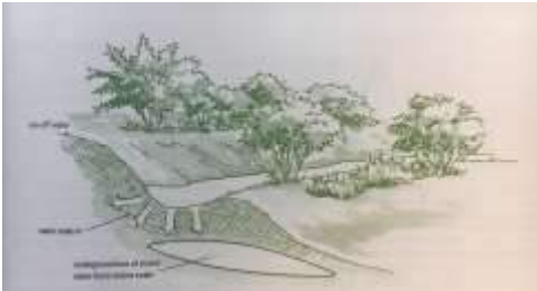
Laid out on contour so water doesn't flow along it, but instead slowly percolates into the soil
